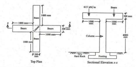
A square column (500 mm  $\times$  500 mm) carries load from two beams, which are mutually perpendicular as shown in figure. Overhang portion of beams carry a total load of 615.0 kN/m (include self-weight). Design the column at top of footing level. Footing is fully embedded in very hard rock. Beams are restrained against rotation at Beam-column junction. The minimum eccentricity is less than 0.05 times the lateral dimension of column. Sketch all details required at column cross-section.
