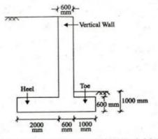
Design and sketch the reinforcement in vertical wall, Toe slab and Heel slab (for maximum Bending moment and maximum shear force only) for the cantilever retaining structure shown in figure. Following parameters may be used for design and sketch :
