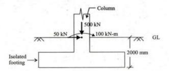
An isolated footing is transferring load from a column (300 mm  $\times$  300 mm) as shown in figure. Arrange the plan dimensions of footing so that there will be uniform soil pressure intensity. Following parameters may be used.
