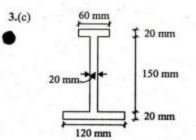
A beam of unsymmetrical I section shown in figure is simply supported over a span of 8 m. It carries a uniformly distributed load of 20 kN/m over the entire span. Draw the sketch for shear stress variation across the depth of the cross-section located at a distance of 3 m from left end A. 20
