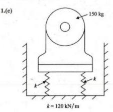
A motor of 150 kg mass is supported by four springs as shown in figure. Each of the springs has a stiffness of 120 kN/m. The unbalance of the rotor is equivalent to a mass of 40 g located at 150 mm from the axis of rotation. The motor is constrained to move vertically. Find
