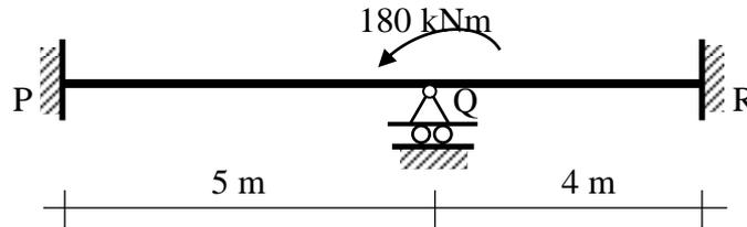
The rotation at Q (in rad, up to two decimal places) is \_\_\_\_\_
