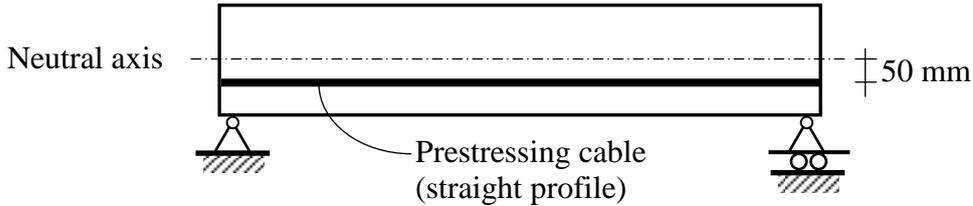
The beam carries a uniformly distributed load of 6 kN/m over its entire span. If the effective flexural rigidity  $EI = 2 \times 10^4 \text{ kNm}^2$  and the effective prestressing force is 200 kN, the net increase in length of the prestressing cable (in mm, up to two decimal places) is \_\_\_\_\_
