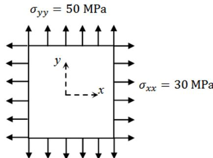
The Young’s modulus of the material is  $2 \times 10^{11} \text{ N/m}^2$  and the Poisson’s ratio is 0.3. If  $\sigma_{zz}$  is negligibly small and assumed to be zero, then the strain  $\epsilon_{zz}$  is
