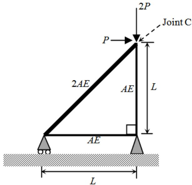
Given that  $E = 2 \times 10^{11} \text{ N/m}^2$ ,  $A = 10 \text{ mm}^2$ ,  $L = 1 \text{ m}$  and  $P = 1 \text{ kN}$ . The horizontal displacement of Joint C (in mm, up to one decimal place) is \_\_\_\_\_
