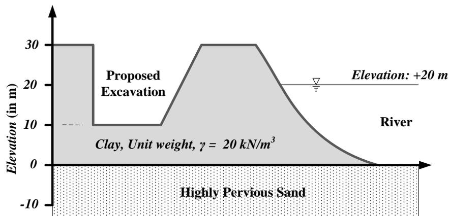
The water level in the adjacent river is at an elevation of +20.0 m. Unit weight of water is  $10 \text{ kN/m}^3$ . The factor of safety (up to two decimal places) against sand boiling for the proposed excavation is \_\_\_\_\_
