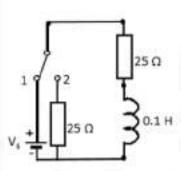
Q.51 In the circuit shown below, the output voltage Vott is \_\_\_\_\_\_ V.
