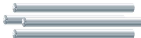
Figure 23: Four rod electrode arrangement commonly used to produce a quadrupole field.
