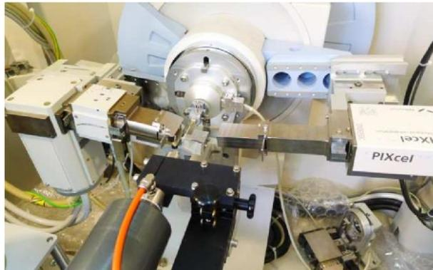
**Figure 13:** Cu  $K\alpha_1$   $\theta/2\theta$  Bragg-Brentano configuration with X'Celerator detector in powder diffractometer PANalytical X'Pert PRO MPD alpha1 at the CCiTUB.
