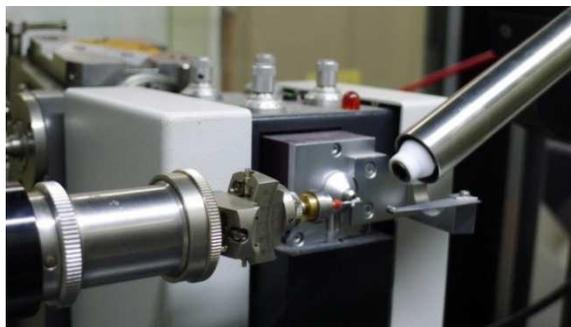
**Figure 1:** Single crystal x-ray diffractometer MAR345 at the CCiTUB. **Figure 2:** Detail of the goniometer and low temperature system in the MAR345 single crystal diffractometer at the CCiTUB
