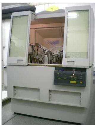
**Figure 11:** X-ray powder diffractometer PANalytical X'Pert PRO MPD alpha1 at the CCiTUB
