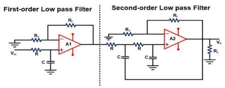
In this figure, the first part shows the first-order lowpass Butterworth filter, and the second part shows the second-order lowpass Butterworth filter.
