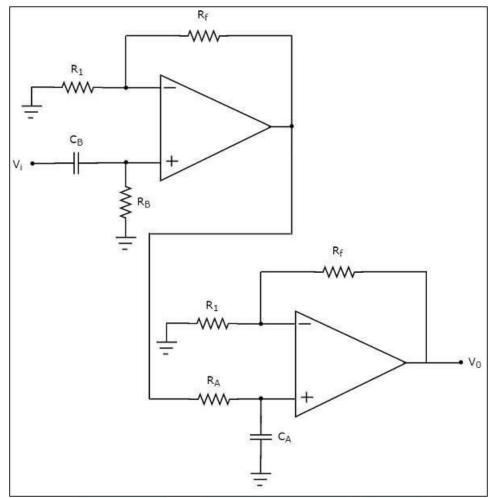
Observe that there are **two parts** in the circuit diagram of active band pass filter:
