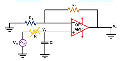
The low pass Butterworth filter is an active Low pass filter as it consists of the op-amp. This op-amp operates on non-inverting mode. Hence, the gain of the filter will decide by the resistor R1 and RF. And the cut-off frequency decides by R and C.
