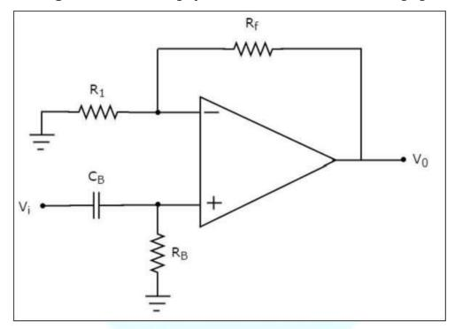
The electric network, which is connected to the non-inverting terminal of an op-amp is a **passive high pass filter**. So, the input of a non-inverting terminal of op-amp is the output of passive high pass filter.
