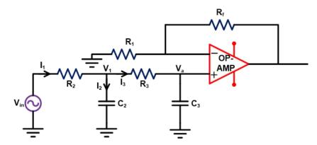
In this type of filter, resistor R and RF are the negative feedback of op-amp. And the cut off frequency of the filter decides by R2, R3, C2, and C3.
