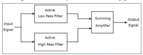
Observe that the block diagram of an active band stop filter consists of two blocks in its first stage: an active low pass filter and an active high pass filter. The outputs of these two blocks are applied as inputs to the block that is present in the second stage. So, the **summing amplifier** produces an output, which is the amplified version of sum of the outputs of the active low pass filter and the active high pass filter.
