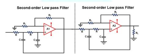
If the gain of both filters is set at 1.586, the voltage gain will be down 6 dB at the cut-off frequency. We can get a flatter response by choosing different values of voltage gain for both stages. According to the advanced research, we get maximum flat response, if we use the voltage gain 1.152 for the first stage and 2.235 for the second stage.
