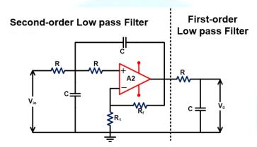
The voltage gain of a second-order filter affects the flatness of frequency response. If the gain of the second-order filter is kept at 1.586, the gain will down 3db for each part. So, the overall gain will down 6dB at the cut off frequency.
