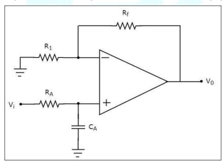
The electric network, which is connected to the non-inverting terminal of an op-amp is a **passive low pass filter**. So, the input of a non-inverting terminal of an op-amp is the output of a passive low pass filter.
