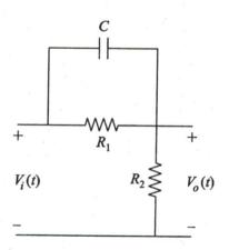
A sinusoidal voltage of 10 V amplitude at 100 Hz is applied to a lead network shown in figure. The phase difference between the input voltage  $V_i(t)$  and output voltage  $V_o(t)$  is 44.43°. If  $C = 0.1~\mu F$  and  $R_1 = 100~k\Omega$ , determine the value of  $R_2$  and the magnitude of steady state output voltage.
