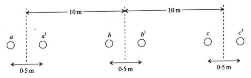
The configuration of a 400 KV 3 phase line is shown in figure. The radius of each sub-conductor is 2 cm. Calculate the charging mega volt-amperes if line is operating at 50 Hz and has a length of 300 km.
