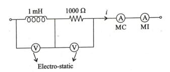
A current of  $(0.5 + 0.3 \sin \omega t - 0.2 \sin 2\omega t)$  amps is passed through the circuit shown in figure. Determine the reading of each instrument if  $\omega = 10^6$  rad/sec.
