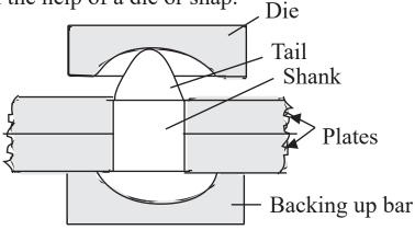
Riverting may be done by hand or riveting machine.
