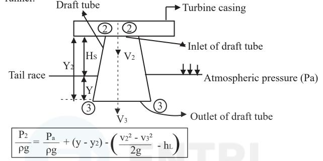
The above equation is valid for the straight conical draft tune shown above. The term  $(y - y_2)$  is called as the suction head of the drafy tube. (Hs). The term  $\left(\frac{V2^2 - V3^2}{2g}\right)$  is called dynamic head.
